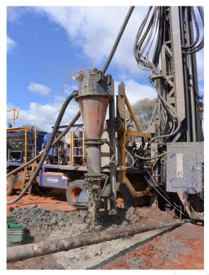
Figure 1: On several holes the volume of brine encountered curtailed drilling speeds. Broad, coarse-sand basal profiles were intersected across the Resource.
