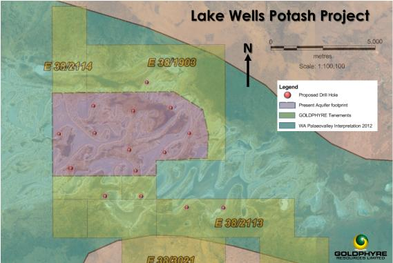
Figure 4: Lake Wells Potash Project, Planned Air-core drilling program
