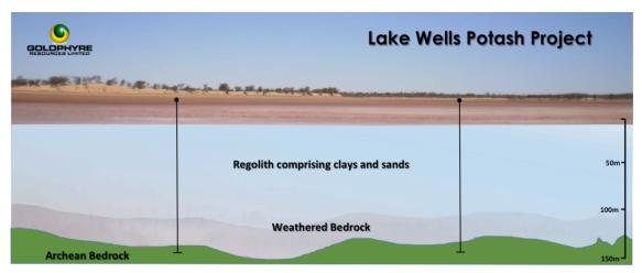
Figure 3: Lake Wells Potash Project, Schematic cross section with proposed drill hole trace demonstrating blade refusal penetration through regolith and deep palaeochannel section
