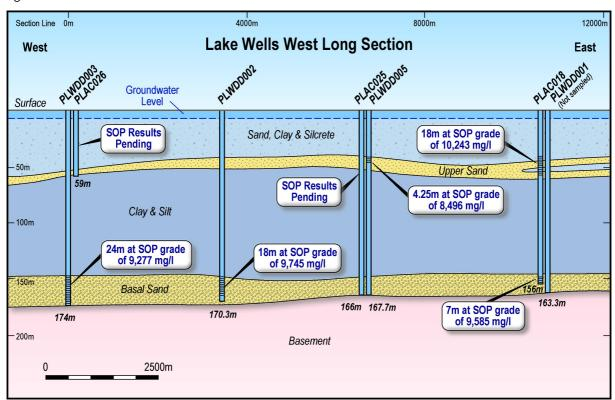
Figure 2: Long section of the western section of the project, showing basal and upper sand intersections
