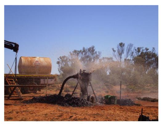
Figure 7: Drilling into the basal sand layer at the Lake Wells Potash Project
