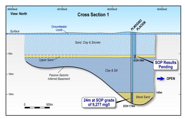
Figure 3: Cross section 1 showing drill holes PLWDD003 and PLAC026, western end of the Project
