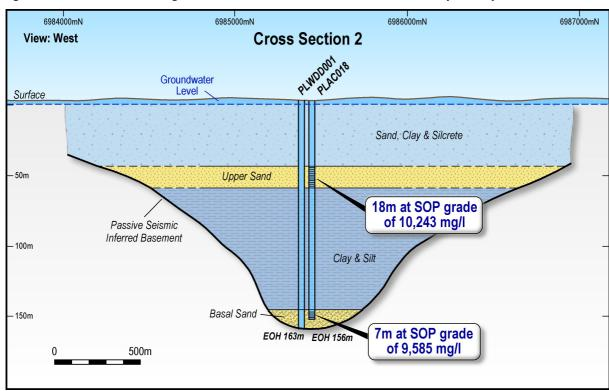
Figure 4: Cross section 2 showing drill holes PLWDD001 and PLAC018, western end of the Project
