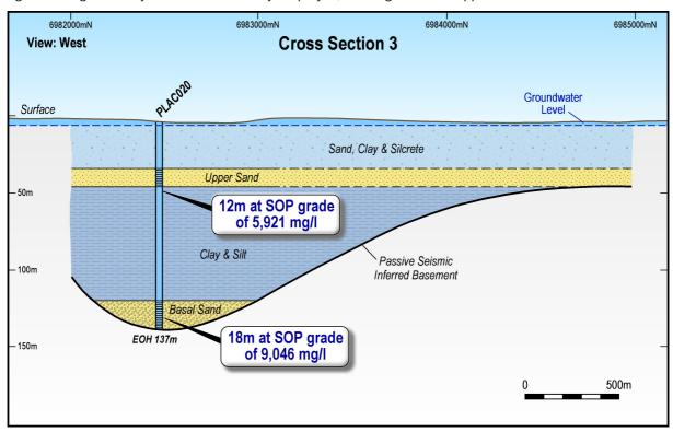
Figure 6: Cross section 3 showing drill hole PLAC020, eastern end of the Project
