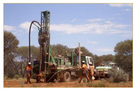
Figure 9. Air Core Drill Rig at Iron Tank Prospect, Mailman Hill
