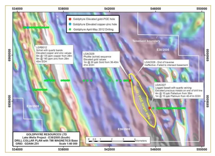
Figure 2. Lake Wells EAST Area (E38/2505) Drill Collar Plan with TMI Magnetics basemap showing elevated gold, PGE, copper and zinc values.
