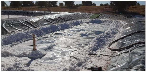
Figure 2: Harvest Pond 1 with stockpiled K and SO4 bearing salts after brine transfer into Harvest Pond 2
