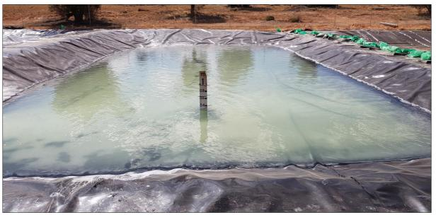
Figure 3: H2 one day after the transfer of concentrated brine from H1 showing immediate K salt crystallisation
