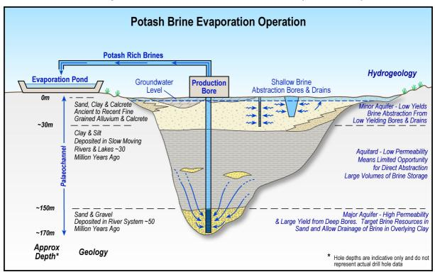
Figure 1: Goldphyre's current diamond drill program is targeting the deepest sections of the extensive palaeovalley, which is where the highly porous basal sand layers are found
