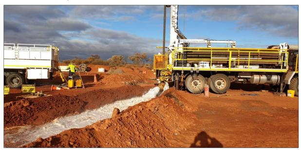
Figure 2: 19LWPR002 was developed through 62 metres of sands including importantly a 33.5m intersection of basal sands which at the Lake Wells SOP project have historically returned very high flow rates
