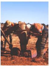
Figure 3: Lake Wells Potash Project, sampling brines out of the cyclone
