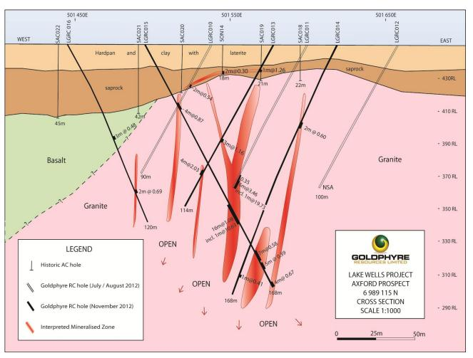
Axford Prospect – Cross Section shows gold mineralised shoots within broad quartz-sulphide alteration zones identified in tonalite/porphyry host<sup>1</sup> similar to new GOR Gruyere gold discovery
