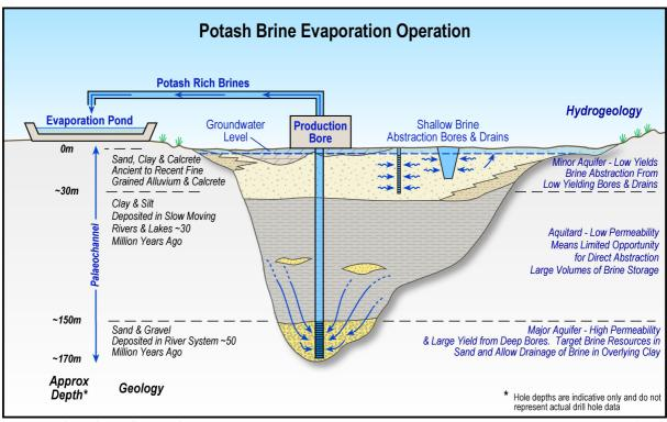
Figure 2: The Lake Wells Potash Project is targeting a 75,000 – 100,000 tpa SOP operation, abstracting potash rich brines from an extensive, deep palaeochannel into evaporation ponds
