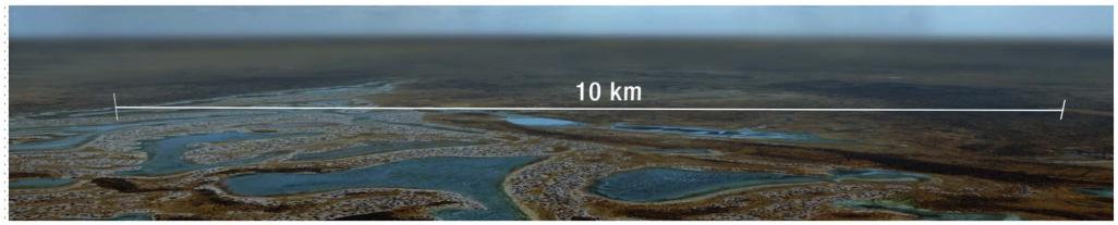
The Lake Wells SOP Project concentration ponds will be built on-lake to take advantage of topographic features and highly-impermeable sub-surface clay layers
