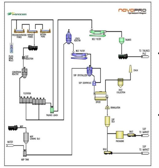
Lake Wells SOP processing plant design including MOP to SOP conversion circuit
