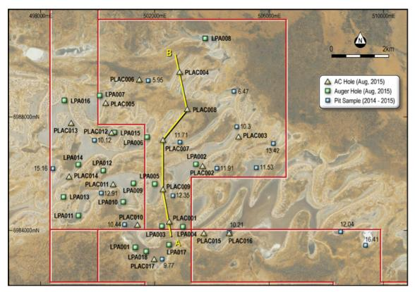
Figure 2: Lake Wells Potash Project, Drill collar location plan showing air-core and auger holes drilled on and off the salt lake surface
