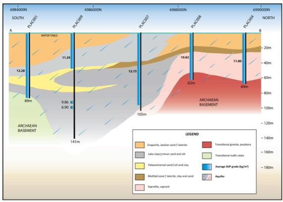
Figure 3: Lake Wells Potash Project, Cross-section showing average down-hole SOP grades and regolith profile
