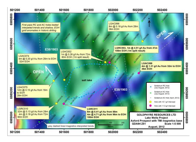
Figure 2. Axford Prospect Drill Collar Plan with gold intercepts and TMI Magnetics base map
