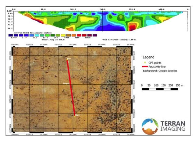
Figure 2: Site E resistivity cross-section and map
