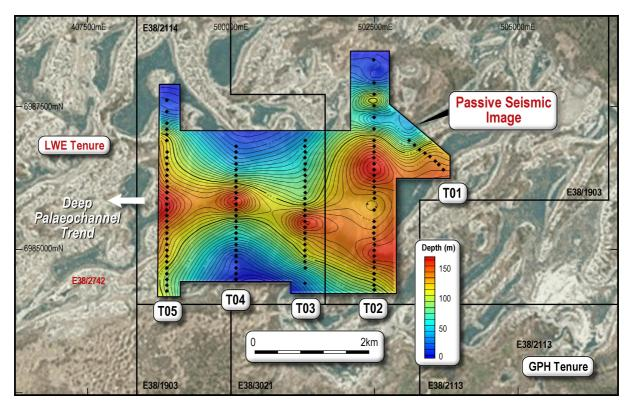
*Figure 2: The seismic program delineated an east-west trending palaeovalley with depths up to 170m*
