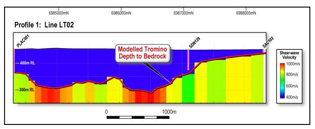
*Figure 7: Line 2, historic drill holes PLAC001, SDN129 & SAC102. It is likely the outlying depth reading to the east of this line is an error due to poor data*
