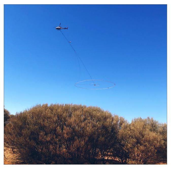
Figure 2: Helicopter-borne VTEM<sup>™</sup> survey in action over the Laverton Downs Project.
