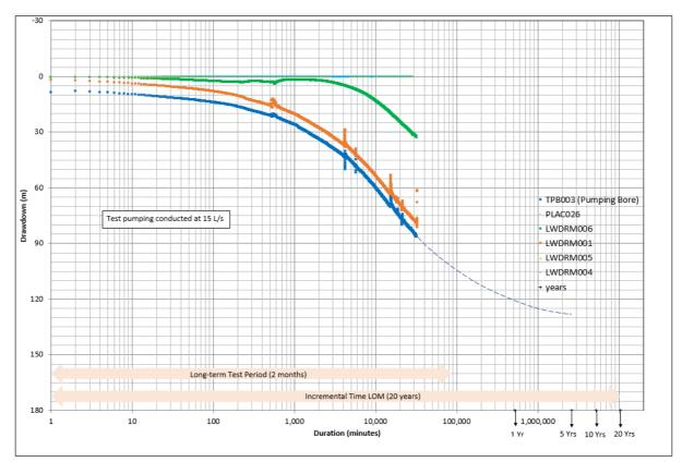
Figure 5: TPB003 Test Pumping Response
