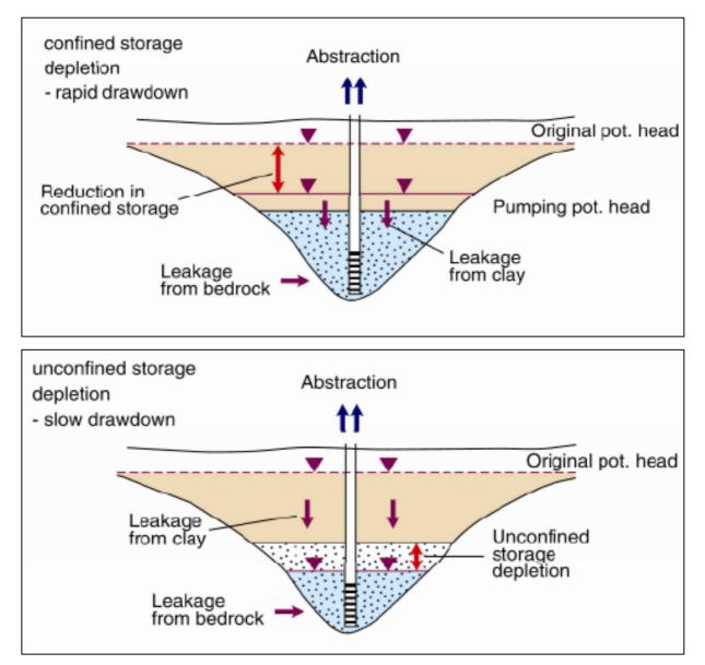
Figure 3: Palaeochannel cross section showing confined and unconfined storage depletion
