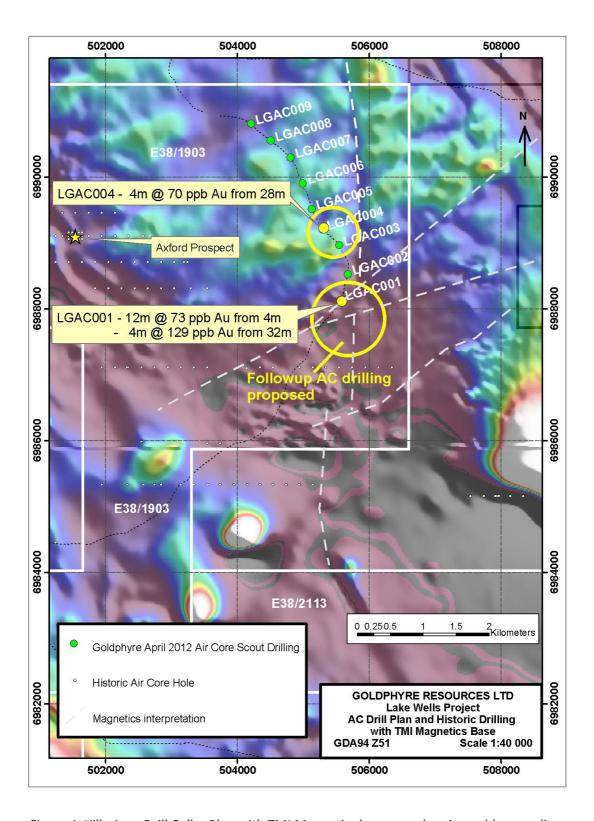
Figure 1. Yilly Area Drill Collar Plan with TMI Magnetics basemap showing gold anomalies.
