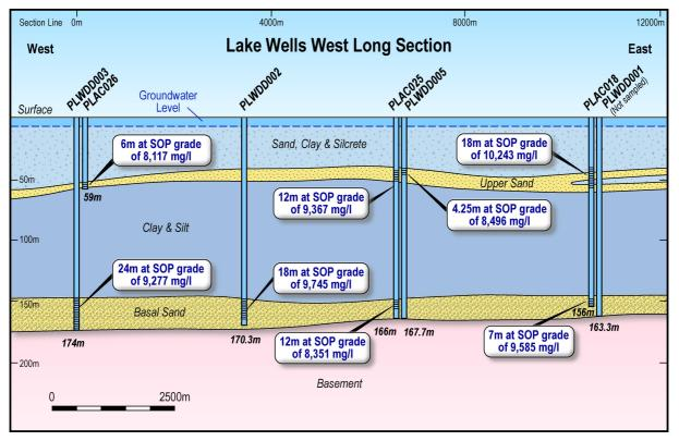
Figure 3: Long section of the western section of the project, showing basal and upper sand intersections
