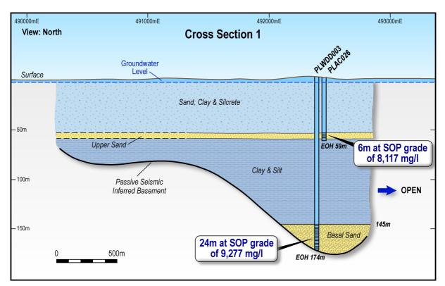
Figure 4: Cross section 1 showing drill holes PLWDD003 and PLAC026, western end of the Project
