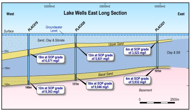
Figure 5: Long section of the eastern section of the project, showing basal and upper sand intersections
