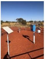
ACP has installed and commissioned a 14 module permanent weather station at the Lake Wells Potash Project. The station is equipped with a remote satellite system, meaning the Company and its consultants are able to collate meteorological data, such as air temperature, barometric pressure and humidity, 24/7. This data will continue to be collected into the life of the project, and feed into the models being built around pond sizing.
