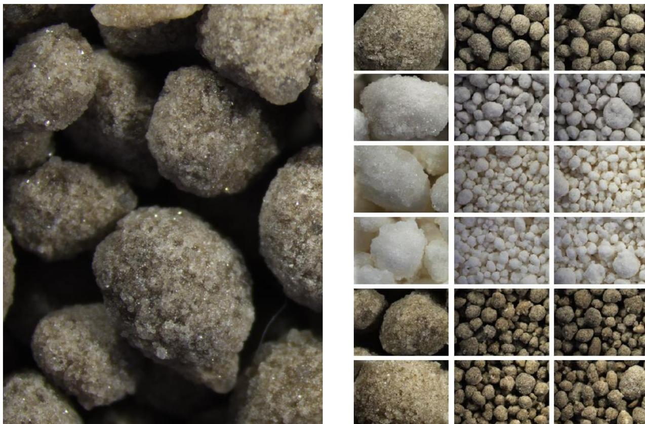
**Figure 1: LSOP granulated product showing well-formed granules**
