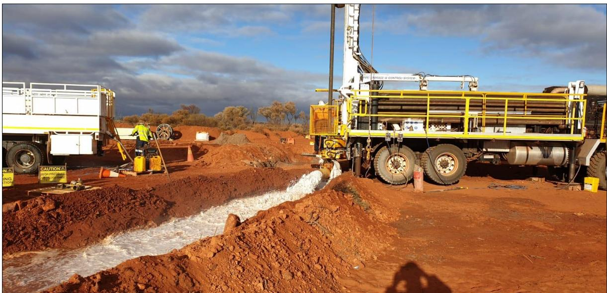
*Figure 2: 19LWPR002 was developed through 62 metres of sands including importantly a 33.5m intersection of basal sands which at the Lake Wells SOP project have historically returned very high flow rates*
