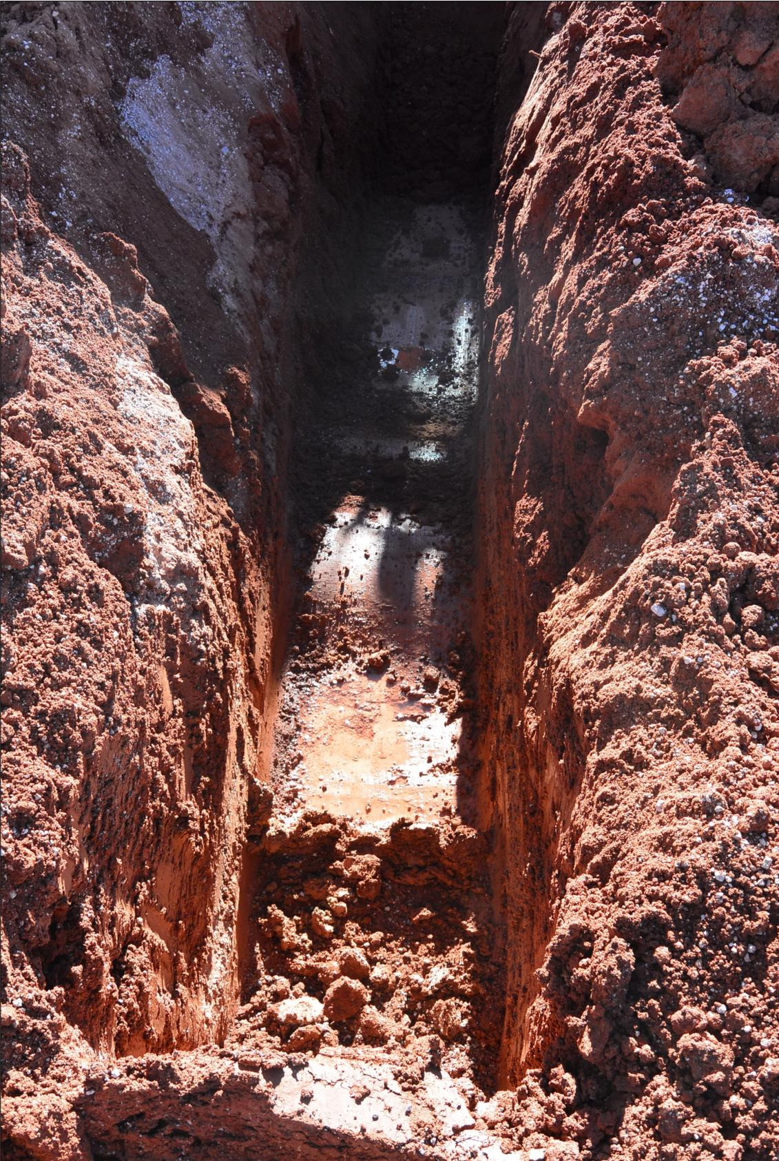
*Figure 4: Surface clays across the playa at APC’s Lake Wells SOP project will allow unlined on-playa concentration ponds to be developed saving significant CAPEX through development*
