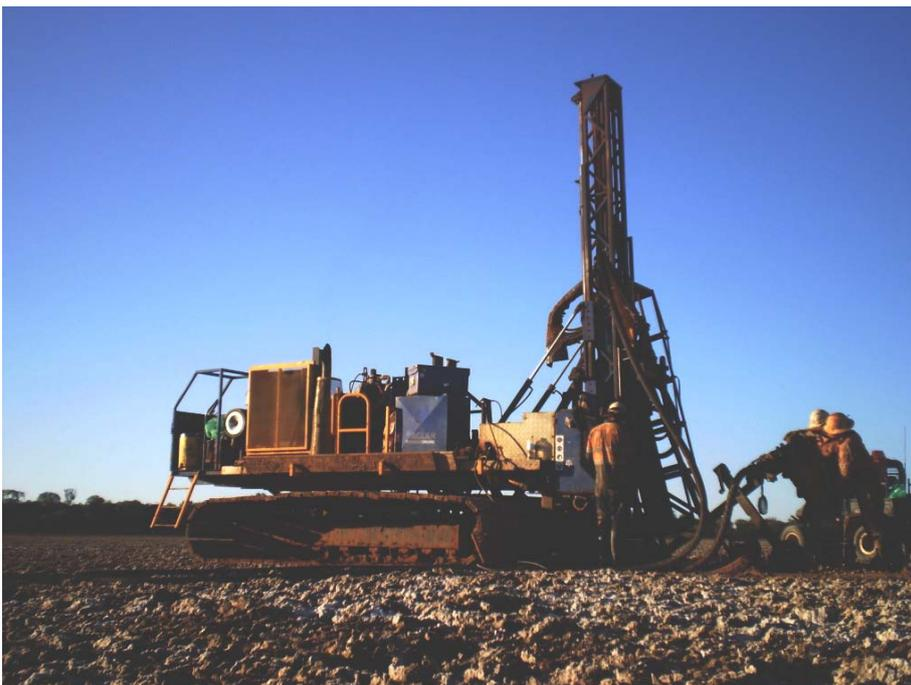
Figure 1: Lake Wells Potash Project, track-mounted AC rig drilling on lake surface
