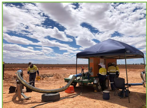
Figure 2: Step rate testing
