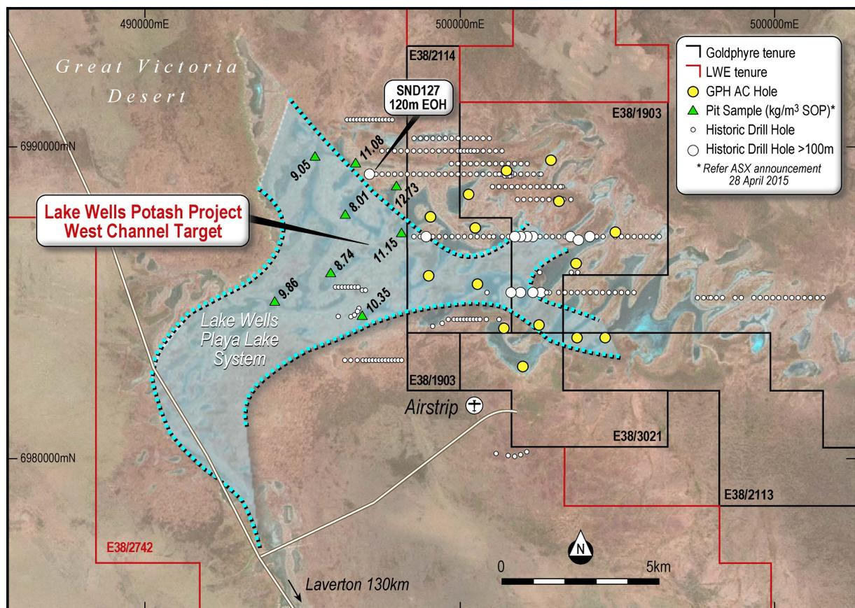
Figure 3: Lake Wells drill & pit sampling location plan showing the West Channel target and palaeovalley trend
