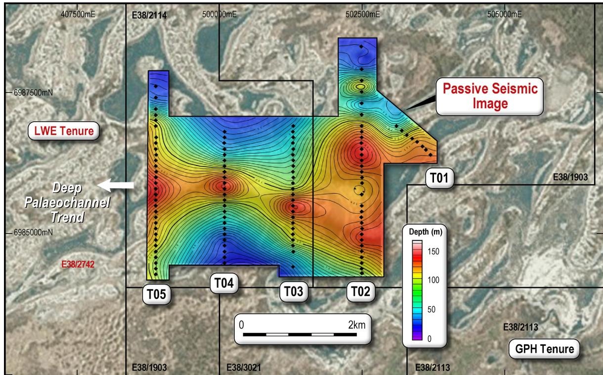
Figure 5: Initial seismic survey modelling indicates a palaeovalley trend extending to the west of the project area, with depths reaching +160 metres
