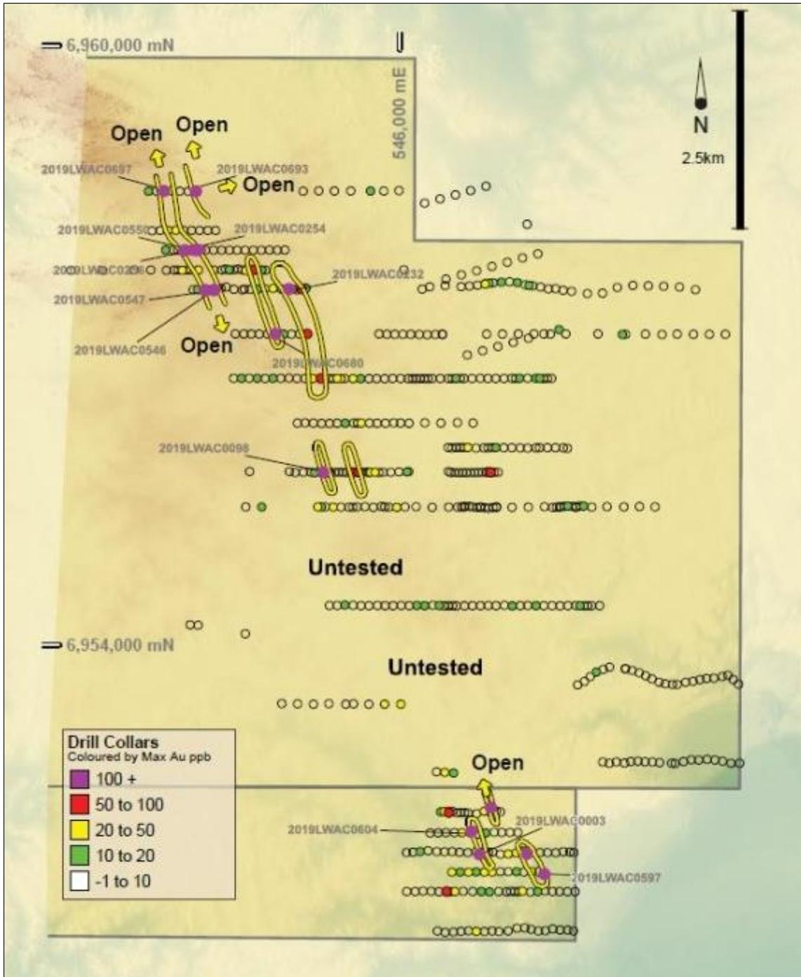
Figure 3: SYAC gold anomalies from aircore drilling. Outlined anomalies are coherent maximum gold in hole anomalies above 50ppb Au
