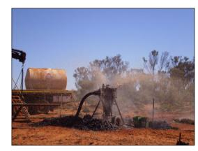
Piercing the clay lithologies into the basal sand aquifer produces high-pressure, hypersaline brine flows
