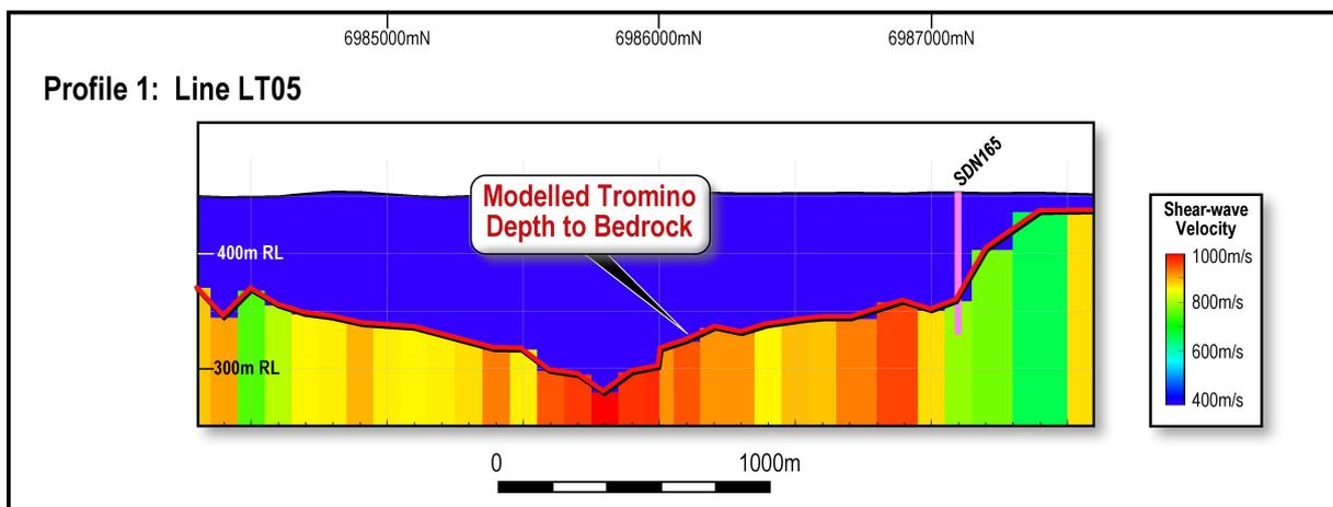
Figure 4: Line 5, the western most survey line & historic drill hole SDN165
