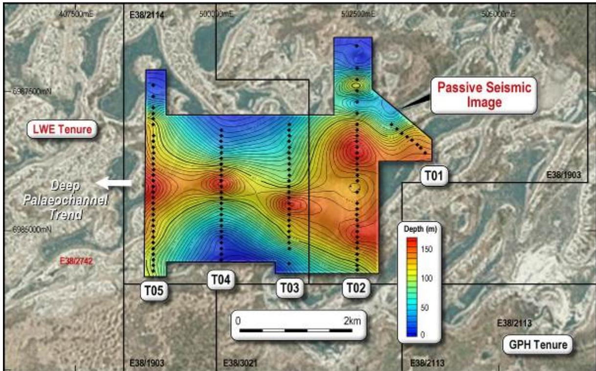
Figure 3: The seismic program delineated an east-west trending palaeovalley with depths up to 170m
