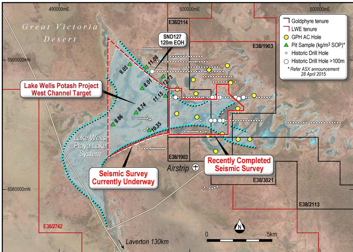
Figure 6: Processing of seismic program is currently underway on the LWE tenure contiguous and to the west of GPH's ground
