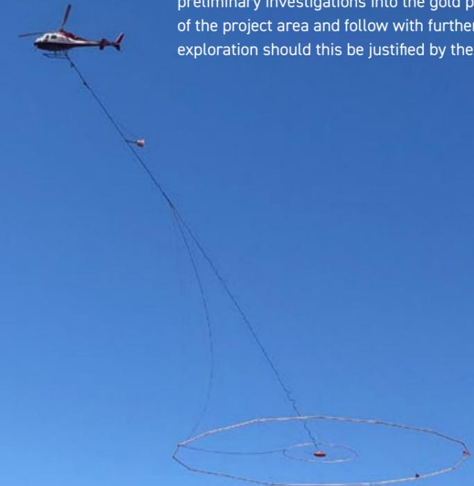
Figure 10: Helicopter-borne VTEM™ survey at the LDP
