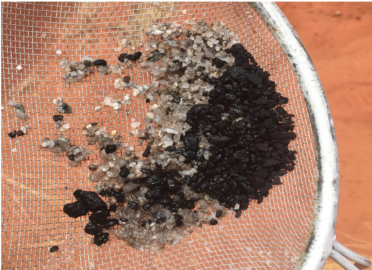
*Figure 3: Example of coarse quartz sand (white) and lignite (black) found in the basal aquifer at the Lake Wells SOP Project. This example is from PLRC021, 150 to 151m below ground level.*
